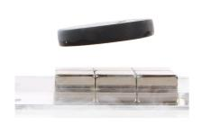
Using the tweezers, gently try to move it in all directions and feel the resistance due to the pinning force. Show that the superconductor can be placed in any orientation including hanging upside down under the magnet matrix..
