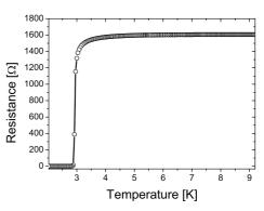
Mercury at low temperatures. He noticed a sudden drop in the resistance below a certain temperature and (boldly) claimed to have found a new state of matter, which was later named 'Superconductivity'.
