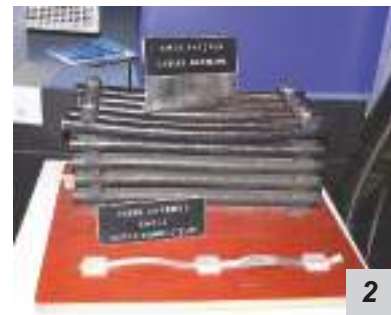
Figure 5: Regular and high temperature superconducting cables for 12,500 amperes used at and Large Hadron in CERN (above and below respectively).
